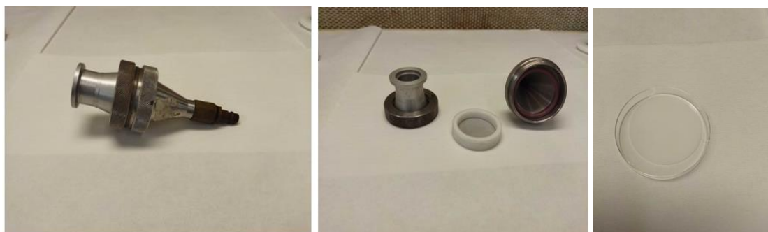
Figure 1: a) Filter holder, b) filter holder and filter cassette, and c) filter material (Nuclepore) for PM 10 sampling
