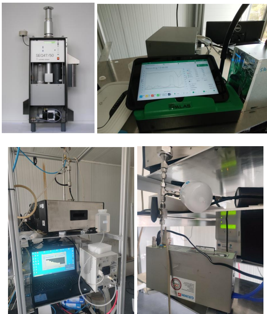
Figure 11: a) PM10 and PM2,5 standard reference sampler (Sven Leckel), b) FIDAS FROG dust monitor, c) Laser Aerosol Spectrometer (LAS, TSI) and d) GRIMM optical particle counter
