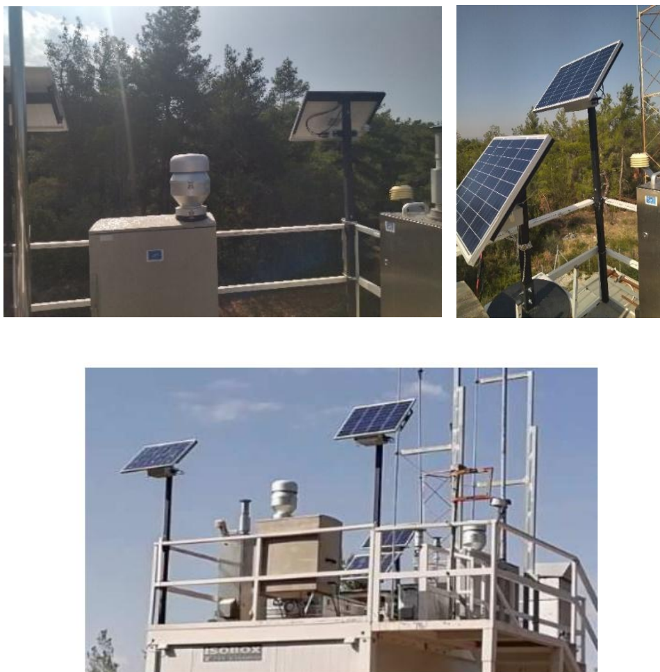
Figure 9: Low-cost sensors, operated with solar panels, are installed at the DEM station for calibration purposes.
