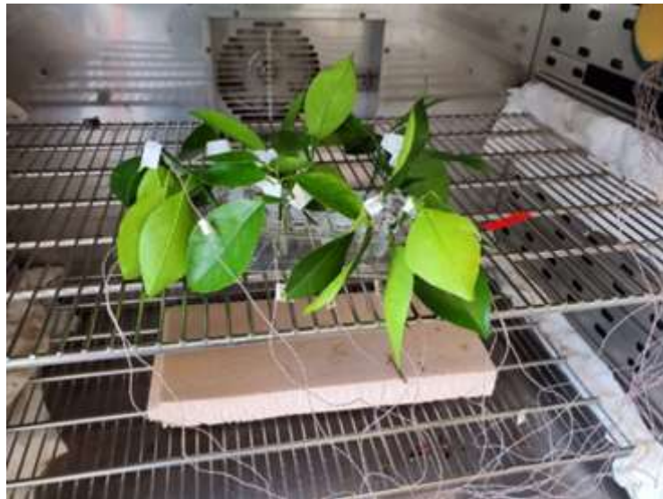
Citrus sinensis equipped with thermocouple inside temperature control chamber (INRAe)
